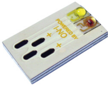
Each LED assembly contains one warm white and one red LUXEON Rebel LED, selected by color bin based on spectral power distribution data from Future Lighting Solutions.
