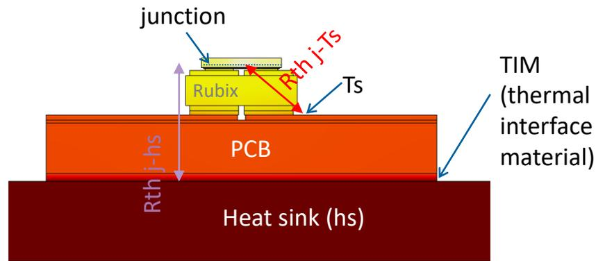
Cross section of the thermal stack
