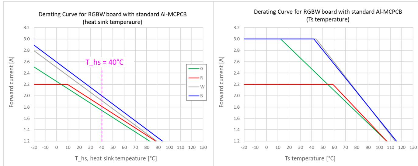
For illustration purpose, at 40°C heat sink temperature, green can be operated at about 1.7A, red at 1.8A, white at 1.9A and blue at 2.0A with standard Al-MCPCB. **We recommend measuring the Ts temperature as this location is clearly defined while heat sink temperature varies spatially depending on the heat sink geometry. See “Typical Rth Table” for typical thermal resistance values to use when doing thermal calculations.**
