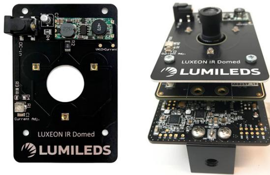
Figure 4. Left: Lumileds IR illumination board with LUXEON IR LEDs. Right: Lumileds board mounted on top of an ON Semiconductor AR0237IRSH00SHRAH3-GEVB kit.
