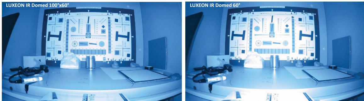
Figure 12. Scene illuminated with 850nm LUXEON IR Asymmetric (left) and 60° emitters (right), showing that an asymmetric illumination prevents overexposure of nearby objects.
