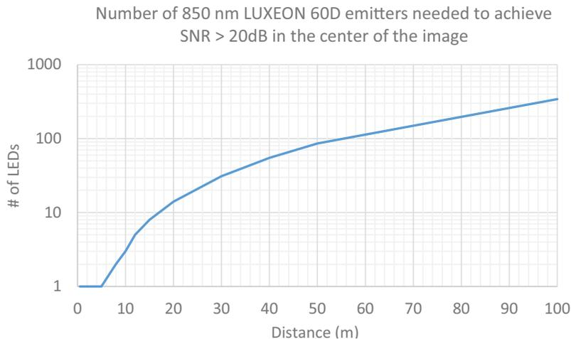
**Figure 15. Number of LUXEON IR 60° 850nm emitters needed to obtain a 20 dB SNR at different distances from the object.**
