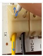
2. To remove wire, insert the tool into the opening and push the tool down and along the blue arrow while pulling the wire away.
