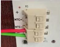
1. Insert stripped wire into the connector holes
