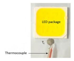
Figure 1. An example of a representative setup of thermocouple (TC) wire attachment via thermal adhesive at the T<sub>c</sub> location.
