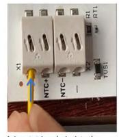
Insert stripped wire into the connector holes until you cannot push further. Do not exert excessive force.
