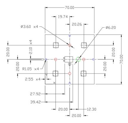
Figure 3. Board mounting screw holes (red circles), optional lens alignment holes (blue semicircle) and a large hole (green circle) for routing power cables through the board.
