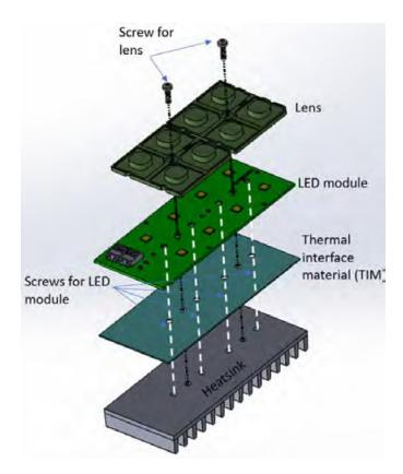
Figure 2. A typical representative of a LED module assembly with heatsink, TIM, lens and screws.
