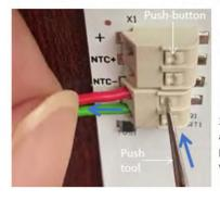
To remove wire, use a suitable push tool and gently apply downward force onto the push-button while simultaneously pulling the wire away from the connectors.
