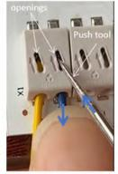
To remove wire, insert the tool into the opening and push the tool along the direction of arrow marking on the connector while pulling the wire away.
