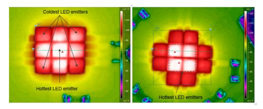
Figure 23. Thermal imaging camera results for LED clusters (150um spacing) with close packing on Al-MCPCB (1oz copper, 3W/(m.K) 100µm dielectric).
