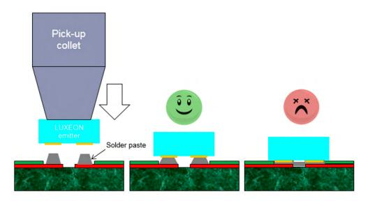
Figure 18. A proper starting point for the mounting z-height of LUXEON HL1Z is 1/3<sup>rd</sup> of the stencil thickness with reference to the top of the stencil paste, i.e. the collet should be in an under-travel position. Center picture shows the optimum result for the collet height setting. Right picture shows over-travel position and may result in bridging of the solder paste on adjacent pads prior to reflow, increasing the likelihood of electrical shorts.
