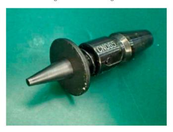
Figure 19. Standard off-the-shelf nozzle "CN065" (inner diameter 0.65mm, outer diameter 1.2mm) with Zirconia tip for Samsung SM421 machine.
