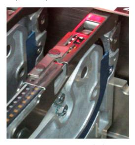
Figure 15. Samsung SM421 feeder.
