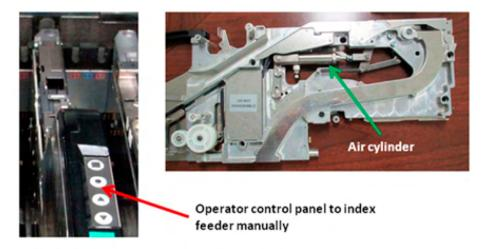
Figure 13. Examples of an electric feeder (left) and a pneumatic feeder (right) which are typically used in pick and place machines to advance the tape with LEDs.
