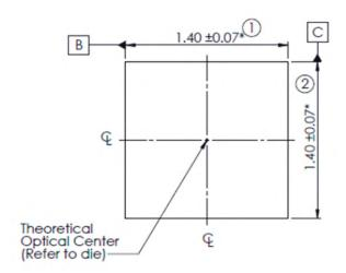
Figure 2. Theoretical optical center is located within the center of the light emitting area. Dimensions in mm.
