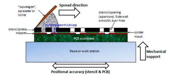
Figure 10. Stencil printing process.
