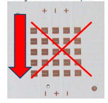
Figure 12. Orientate the PCB such that the stencil printing direction is along the long side of the pads.
