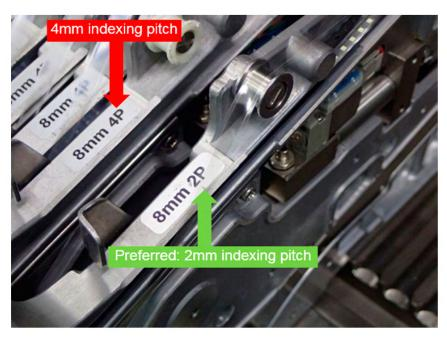
Figure 16. An example of Samsung SM421 feeder with 2mm and 4mm indexing pitches.
