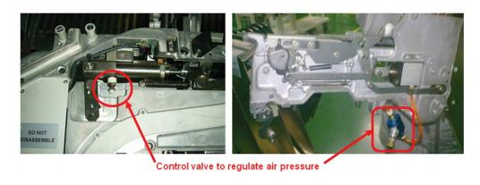
Figure 17. Pneumatic feeder with integrated air pressure control valve (left) and pneumatic feeder with air pressure control valve installed afterwards (right).
