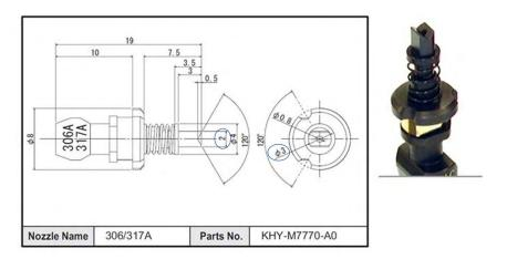
Figure 6. An example of a nozzle with outer size of 2mm x 3mm as shown on the left drawing. See the circled dimensions. Right image is the actual nozzle tip. Dimensions in mm.
