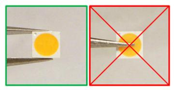
Figure 2. Illustration example of correct handling (left) and incorrect handling (right) of the LUXEON emitter.
