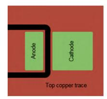
Figure 4. The top copper trace pattern is created such as to maximize the amount of copper surrounding the cathode pad. The green area represents the solder mask opening and the red area represents the top copper layer.
