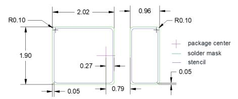
Figure 3. Recommended PCB footprint design for the LUXEON 2835 Commercial (dimensions are in millimeters).
