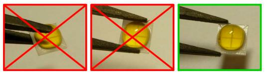
Figure 3. Incorrect handling (left and middle) and correct handling (right) of LUXEON emitters.
