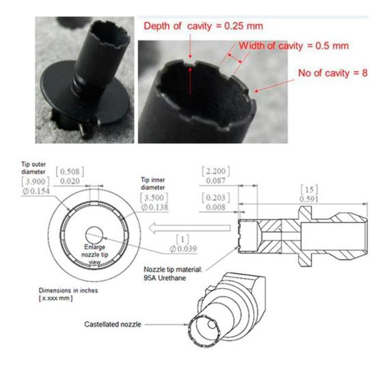
Figure 22. Pictures of castellated nozzle to prevent LUXEON T/TX from getting stuck to the nozzle tip during pick and place process. Below is the drawing of a castellated nozzle for Yamaha YV100X. Drawing courtesy of Count on Tools Inc.
