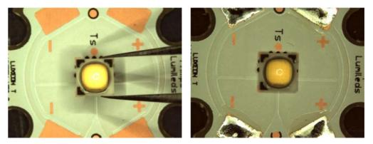
Figure 15. Manual placement of a LUXEON emitter onto a PCB (left). Self-alignment during reflow yields, in most cases, adequate placement accuracy (right) for manually placed LUXEON emitters.
