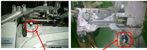
Control valve to regulate air pressure
