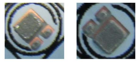
Figure 10. A poorly placed stencil may cause some of the solder paste to be deposited onto the solder mask, reducing the amount of solder paste which is available on the pads to establish a strong solder joint. In this example, the silk screened circles within the LUXEON package outline may also lift the stencil from the solder mask, compromising the quality of the solder paste deposition process.
