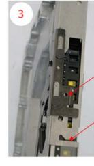
The shutter moves forward and backward during indexing.
