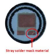
Figure 33. Examples of poor PCB workmanship which may adversely impact the solder joint between the PCB and the LUXEON emitter.
