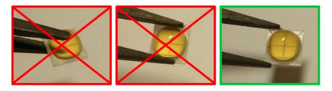
Figure 3. Incorrect handling (left & middle) and correct handling (right) of a domed LED package similar to LUXEON V.
