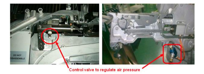
Figure 17. Pneumatic feeder with integrated air pressure control valve (left) and modification made to the pneumatic feeder by installing air pressure control valve (right).
