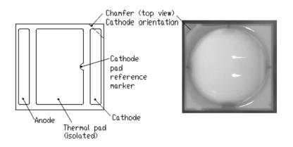
Figure 1. Bottom view (left) and top view (right) of the LUXEON V LED.
