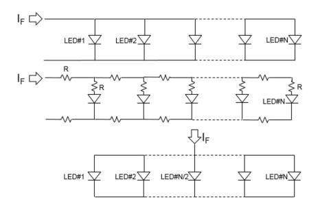
Figure 6. Effect of trace resistance and routing pattern on LED light output performance as described.
