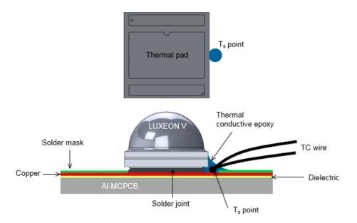
Figure 8. Drawings showing the recommended location of the T<sub>s</sub> point (top).
