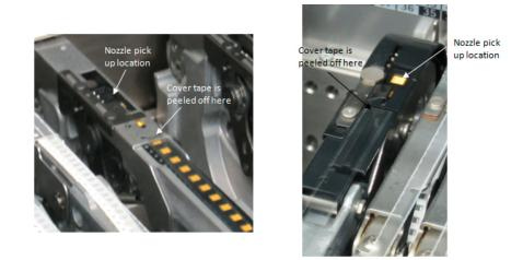
Figure 14. Examples of Samsung SM421 (left) and Juki KE-2080L (right) pick and place feeders used to pick and place LUXEON domed packages.
