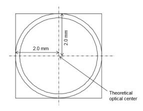
Figure 2. The theoretical optical center of LUXEON V.
