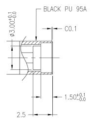
Figure 9. Generic nozzle's tip design. Outside diameter is 4.2mm and interior diameter is 3.8mm. All dimensions are in millimeters.
