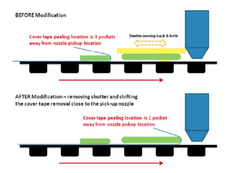
Figure 15. Illustration of the general principle behind the feeder modification where, in some cases, there may be a need for the LED emitter to be picked up immediately after the cover tape is peeled off.
