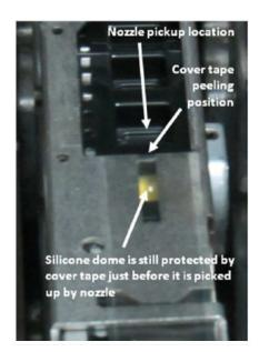
Figure 16. An actual example of a modified feeder, which protects the LED silicone dome with cover tape still on prior to pick up.
