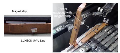
Figure 10. LUXEON UV U Line is held by the magnet strip (left). Feeder (e.g. Panasonic CM402) equipped with magnet strip (right).
