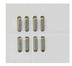
Figure 6. An example of good stencil printing on 4-up MCPCB star board.
