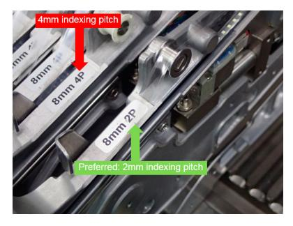
Figure 11. An example of Samsung SM421 feeder with 2mm (preferred) and 4mm indexing pitches.
