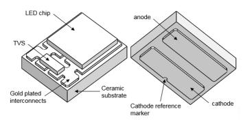
Figure 1. 3D renditions of a representative of LUXEON UV U Line. Top view (left) and bottom view (right).
