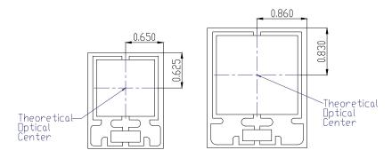
Figure 2. The optical centers of the LUXEON UV U Line emitter (in mm).
