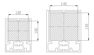
Figure 7. Pick-up area (shaded) for LUXEON UV U1(left) and LUXEON UV U2 (right). Dimensions in mm.
