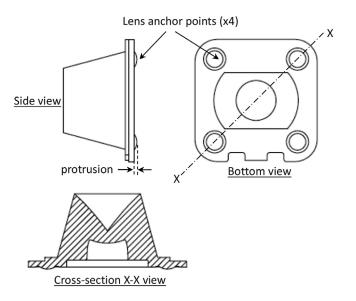
Figure 4. An example of a lens design without "feet." The depth of the PCB required to accommodate these anchor points is labeled as protrusion. It should also include the glue bond line thickness.
