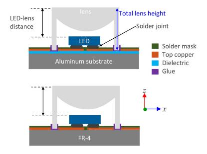
Figure 3. Top drawing represents cross-section of the lens feet on Al-MCPCB. Bottom drawing represents FR-4 PCB where the lens feet are attached to the FR-4 substrate. Drawings are not to scale.
