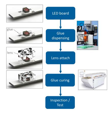
Figure 1. Typical lens attach process flow.
