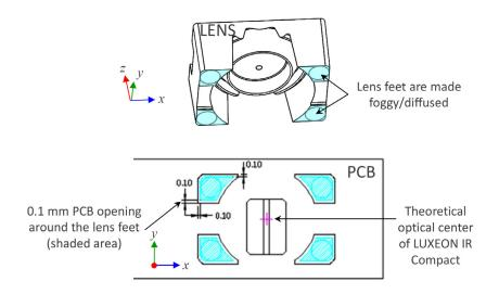
Figure 2. An example of PCB lens feet opening clearance. Top drawing is the lens with lens feet that are foggy/diffused to improve machine pattern recognition. Bottom drawing is the PCB. All dimensions are in millimeters.
