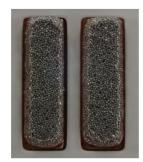
Figure 8. An example of a good stencil printing on PCB.
