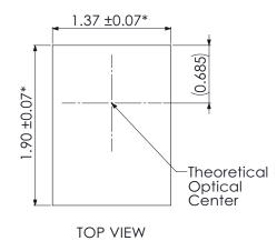
Figure 3. The optical center of LUXEON IR Compact is 0.685mm from the top and 0.685mm from the side edges.
