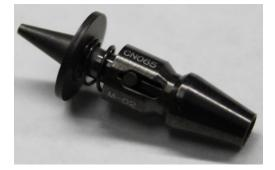
Samsung off-the-shelf nozzle model: CN065 Nozzle tip material: Ceramic (Zirconia) Nozzle inner diameter: 0.65mm Nozzle outer diameter: 1.20mm
