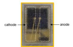
Figure 2. Polarity orientation when viewed from package top. White dashed line are the pad outlines as seen from the top.
