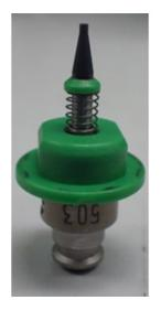
Juki off-the-shelf nozzle model: "503" Nozzle tip material: ceramic (zirconia) Nozzle inner diameter: 0.6 mm Nozzle outer diameter: 1.0 mm
