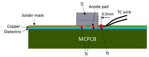
Figure 7. The recommended temperature measurement point Ts is located on the anode copper layer of the PCB, 0.5mm away from the package. The picture above shows an example where to place the welding tip of the thermocouple wire prior to dispensing any thermal conductive epoxy to secure the thermocouple wire.
