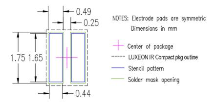
Figure 6. Recommended PCB Footprint for LUXEON IR Compact.
