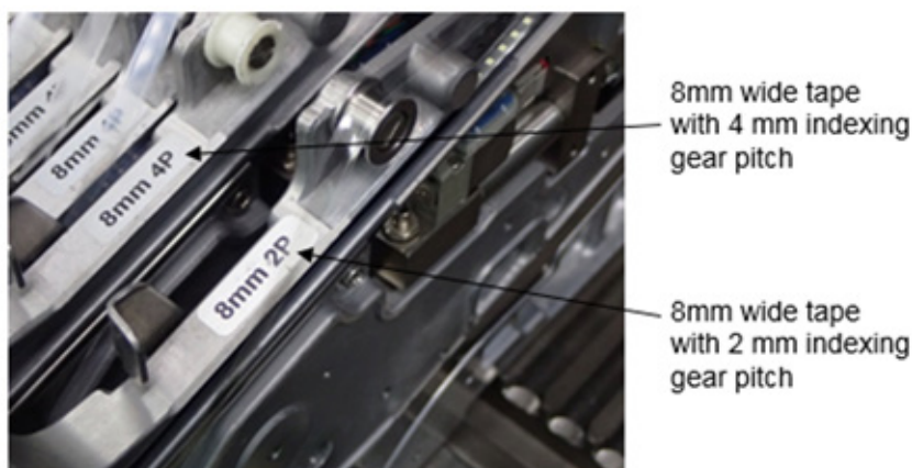
Figure 21. Example of 8mm width tape with 4mm and 2mm indexing gear pitch. Same principle for 12mm width tape.
