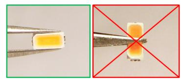
Figure 2. Correct handling (left) and incorrect handling (right) of LUXEON emitters.
