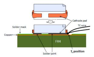
Figure 4. The recommended temperature measurement point Ts is located on the cathode copper layer of the PCB, closest to the package, partially touching the cathode pin. The picture above shows where to place the welding tip of the TC wire prior to dispensing any thermal conductive epoxy to secure the TC wire.
