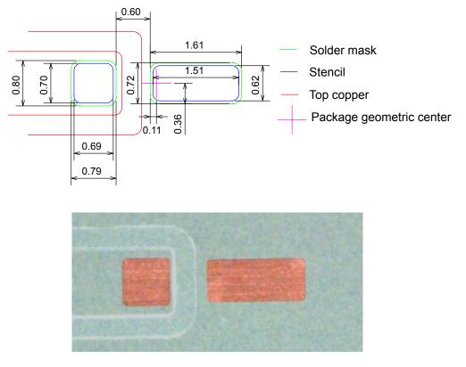
Figure 3. Recommended PCB footprint design for the LUXEON emitter (top). In order to ensure proper heat dissipation from the package electrodes to the PCB, it is best to extend the top copper layer of the PCB several millimeters beyond the package of the LUXEON emitter. See Section 3 for more information on the copper layout. All dimensions are in mm. Bottom picture shows the actual FR4 PCB footprint layout.
