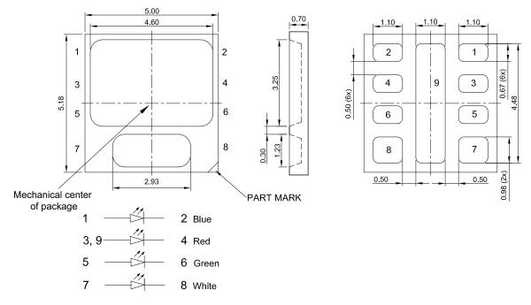
Figure 1. Mechanical Drawing of LUXEON 5052 RGBW.
