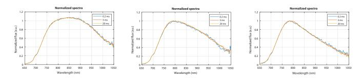
Figure 12. Normalized output spectra of LUXEON IR ONYX at different pulse lengths. Case temperature: left = 25°C, center = 55°C and right = 85°C. Spectra are normalized to their value at 790nm, in order to make shape comparison easier.
