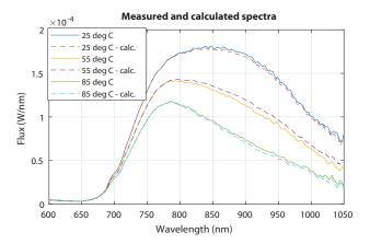
Figure 14. Left: example of linear fitting measured data at 3 different wavelengths (full lines–measured flux at each wavelength, dashed lines–linear fit). Right: Measured (full lines) and calculated based on the linear fit (dashed lines) spectral output of LUXEON IR ONYX at different ambient/case temperatures. Drive current = 350mA.
