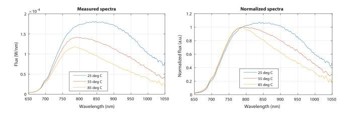
Figure 10. Output spectrum of LUXEON IR ONYX at different case temperatures. Drive current = 350mA. Left: Measured spectra. Right: Spectra normalized to their value at 790nm, in order to make shape comparison easier.
