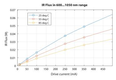
Figure 9. IR flux output of LUXEON IR ONYX vs. drive current at different case temperatures.
