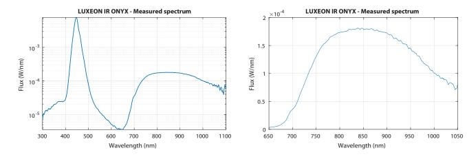
Figure 8. Typical output spectrum of the LUXEON IR ONYX broadband emitter at 350mA drive current and 25°C case temperature. Left: Full spectrm on log scale, including blue light. Right: IR spectrum.
