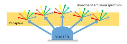
Figure 6. Working principle of a broadband LED emitter; a blue LED is used to pump a phosphor, which emits a wide spectrum. Some of the original blue light also goes through.
