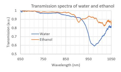
Figure 15. Transmission of water and ethanol, measured using an LUXEON IR ONYX emitter as light source. Optical path length through the liquid: 1cm. Spectra were normalized to transmission value at 670nm.
