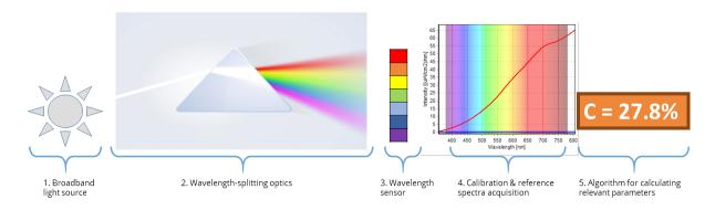
Figure 5. The main building blocks of a spectrometry setup.
