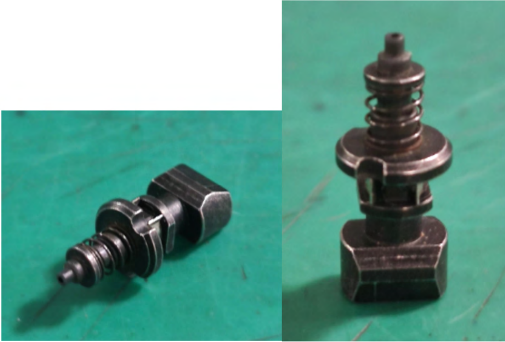
Figure 20: Yamaha Nozzle 309A (KHN-M7790-A1X) with inner diameter 0.7mm and outer diameter 1.2mm with Teflon tip.
