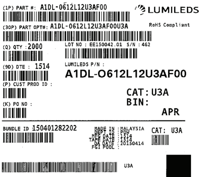
Figure 13. Example of a moisture barrier bag label
