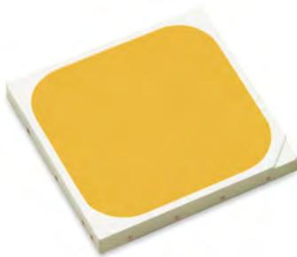
LUXEON 7070 is a multi-die, high power package that provides high luminance from a super robust package to enable cost effective, single optic and directional fixture designs. LUXEON 7070 uses an industry standard 7070 surface mount package with a small Light Emitting Surface (LES). LUXEON 7070 is offered in 70, 80, 90 CRI with a wide range of CCTs, and offers hot-color targeting to ensure that the LEDs are within color target at application conditions of 85°C.
