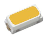
LUXEON 3014 has a compact package size of 3.0mm x 1.4mm x 0.70mm—ideal for achieving uniform light output where space is limited, such as linear applications, tube lighting, and signage. LUXEON 3014 is hot-color targeted at a junction temperature of 65°C, ensuring color consistency and meeting ANSI standards at operating conditions.
