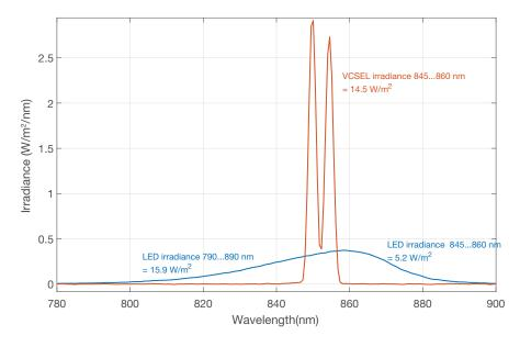
Figure 11. Irradiance of 860nm VCSEL and LED emitters (modulation frequency 20MHz, burst length 400μs), measured at a distance of 0.5m.
