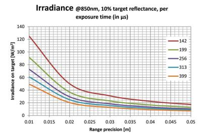
Figure 3. Irradiance on target required to reach a certain precision for Melexis EVK75024 TOF system, at different exposure times/burst lengths. Note: Irradiance values shown here correspond to average irradiance within a burst.
