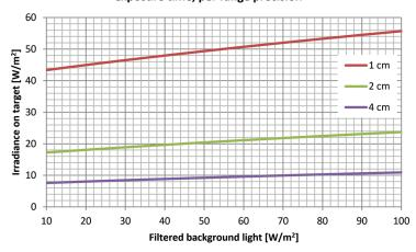
Figure 5. Irradiance on target required to reach different measurement precision values (1, 2 and 4cm respectively) as a function of filtered ambient background light levels. Note: Irradiance values shown here correspond to average irradiance within a burst.
