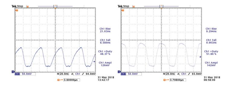
Figure 13. Pulsed behavior of a LUXEON L110 – 0940xxx emitter without (left) and with voltage booster circuit (right).
