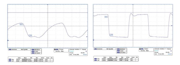
Figure 12. Pulsed behavior of a LUXEON L1I0 – 0940xxx emitter in a Melexis TOF evaluation kit (left) vs VCSEL (right).
