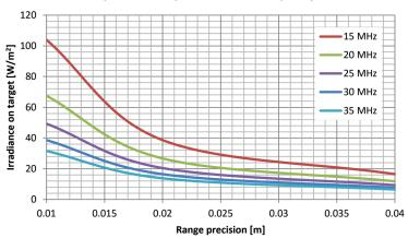
Figure 4. Irradiance on target required to reach a certain precision for different modulation frequencies lengths.
